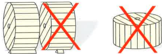
Do not lay drums flat on their sides, use proper stops to prevent drums rolling.
